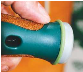
▲ The plastic striking cap has a rubber shock absorption washer below it
